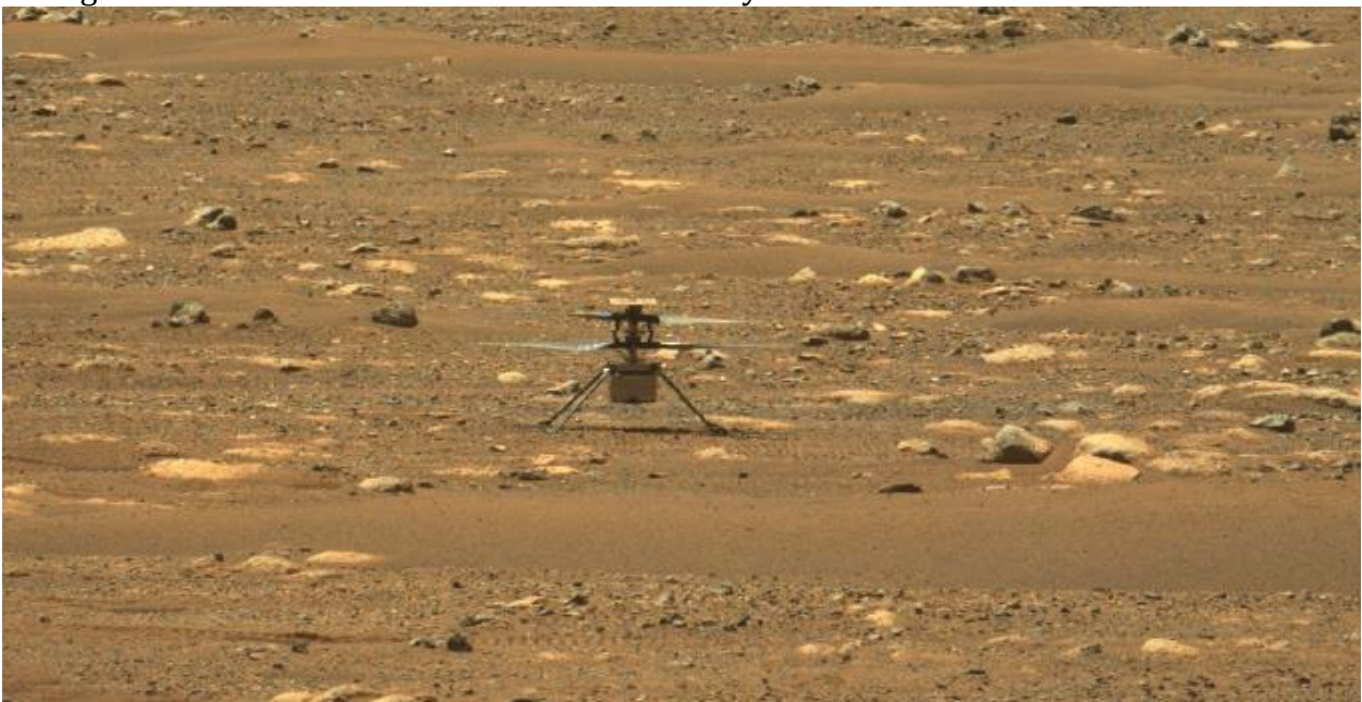
Almost 45 years later, the small helicopter Ingenuity landed with the Perseverance rover and became the first robot to fly in the thin Martian atmosphere. Its blades span 1.2 meters. JPL-CALTECH/NASA, ARIZONA STATE UNIV.
